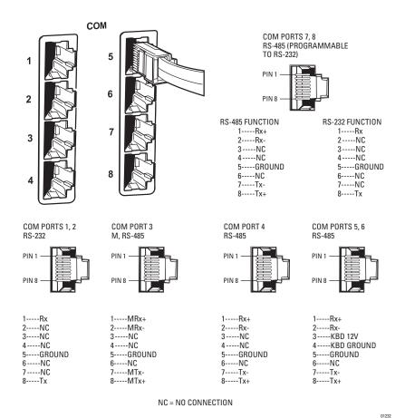
Figure 9. COM Port Connections and RJ-45 Connector Pin-Outs
